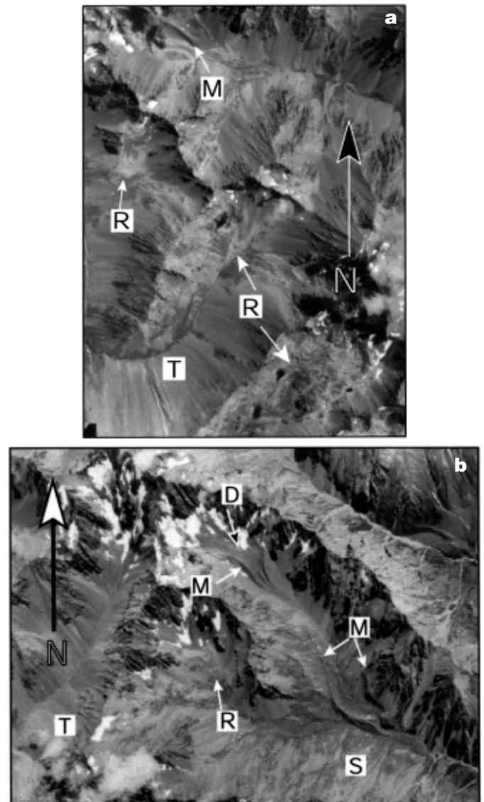
**Fig. 4.** a, Aerial photograph (SN 8595, G/14) showing glacial deposits (M = moraine), active rock glaciers (R) and active talus fans (T) in part of Ben Ohau Range; b, aerial photograph (SN 8595, G/14) showing debris-mantled glaciers (D), active talus fans, moraines (M), snow avalanche tracks (S) and active rock glacier (R) in central Ben Ohau Range.
