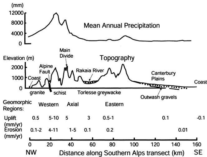
Fig. 2. Cross section through the central Southern Alps, New Zealand, showing mean annual precipitation, uplift and erosion rates. Modified from Whitehouse.<sup>6</sup>
